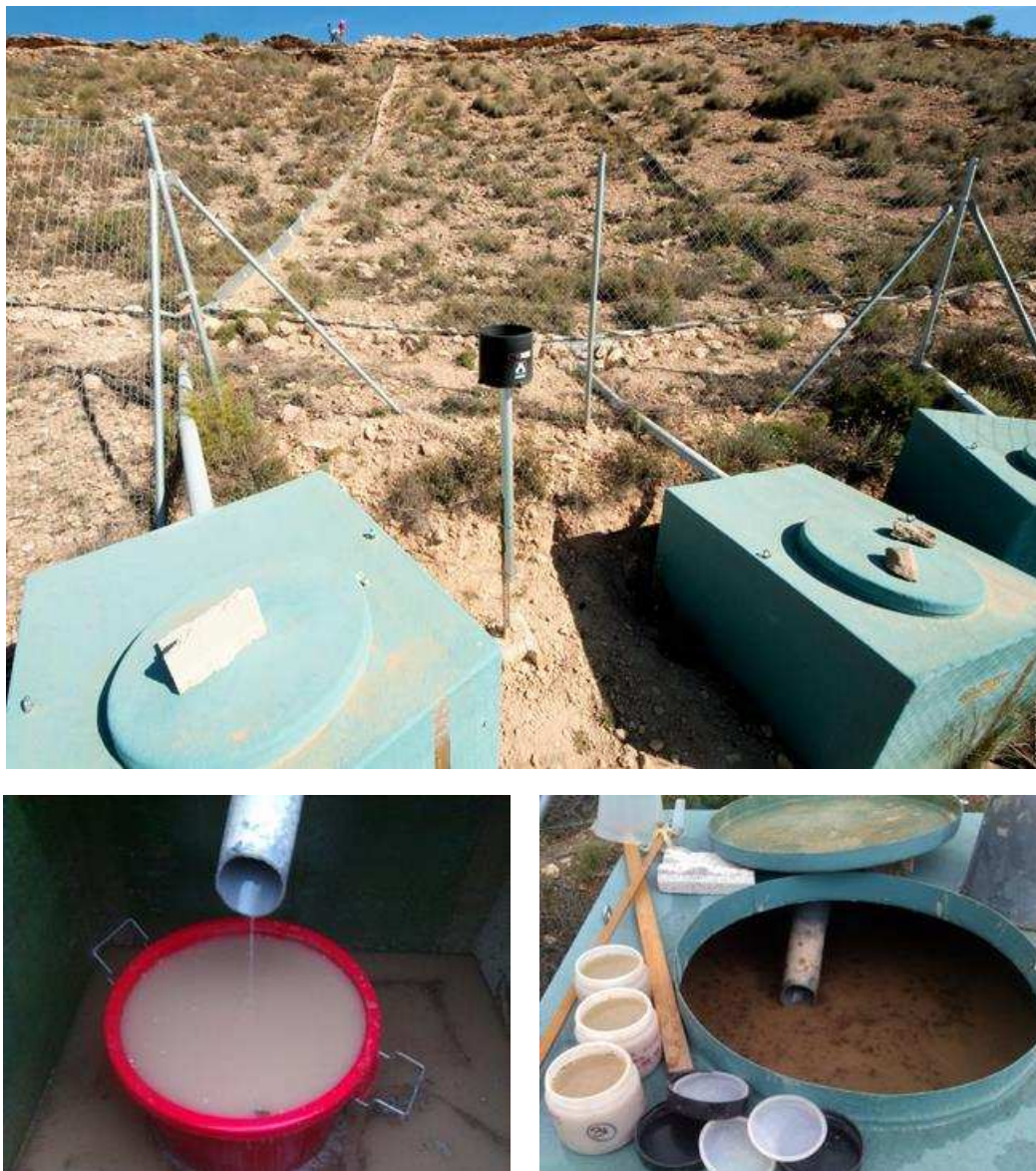
Figure 5. General view of the plots and the containers for runoff and sediment measurements (top) and details of measurement containers after a large rainfall event.
