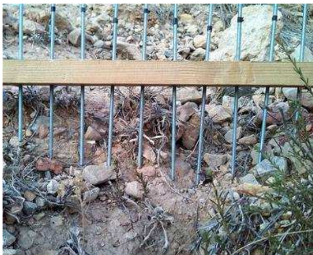
Figure 6. Two-dimensional microprofilometer used for the monitoring of the shape of the rills developed on the experimental plots.
