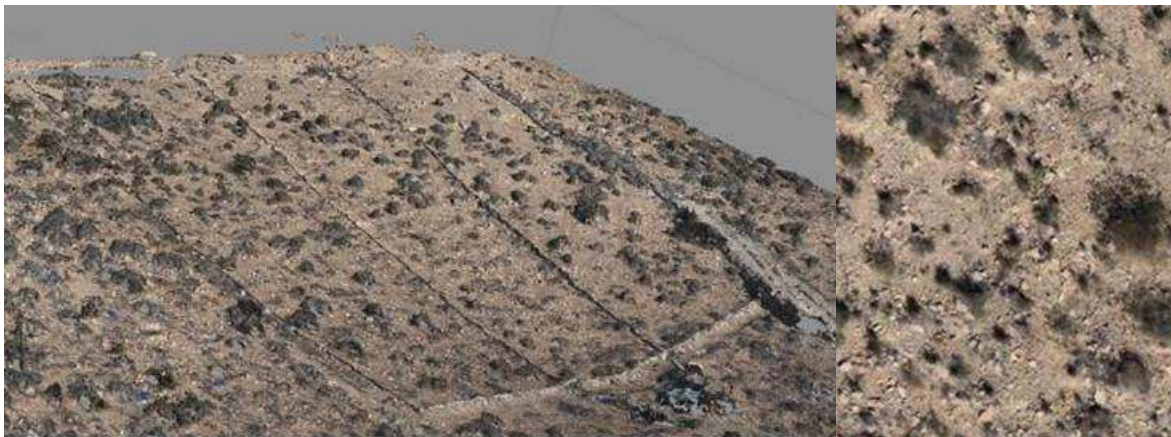
Figure 3. 3D-Image of the experimental slope and plots (left) after treatment (vegetation removal) application, and detail of the soil surface (right).
